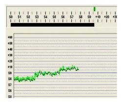
From these observations, it seems that the prototype dipole offers a 6 (or somewhat more) decibel gain over the Wolf River coils configured as a dipole and terminated with 102" whips. 6 dB equates to one S-unit.
