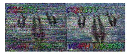
A good signal was received from Jerry W5BKV out of Tulsa, Oklahoma from a distance of 685 miles and bearing of 217 degrees. The measured picture quality at 0349 UTC for the prototype dipole was 70.66%, and 86.07% for the standard Wolf River dipole.
