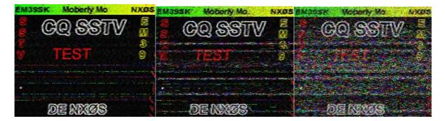
I asked Gary KB9AIT, one of the owners of Wolf River Coils, to transmit an SSTV signal. This comes via ground wave from his QTH only 9 miles away at 173 degrees. The measured picture quality at 2114 UTC for the prototype dipole was 65.23%, and 48.27% for the standard Wolf River dipole.
