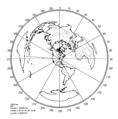
For any two points on the surface of a sphere there is a <u>unique</u> great circle through those two points. For amateur radio use, we can conveniently define these locations as grid squares. This makes it easy to utilize software to determine beam headings to and from two ham QTHs. I use WinGrid 4.1 created by Stacey W4SM to make calculations.
