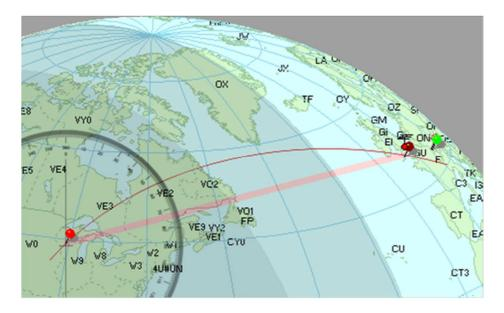
Note that while I can find the long path route to G7SLL simply by subtracting the 3,835 mile short path from 24,854 miles, I CANNOT determine his beam heading simply by adding 180 degrees to my 49.2 beam heading. (If one is at the equator pointing east at 90 degrees, then adding 180 degrees would be correct to calculate the opposite beam heading of 270 degrees.) The Great Circle calculation instead calls for a 299.7 degree heading towards me from his QTH.
