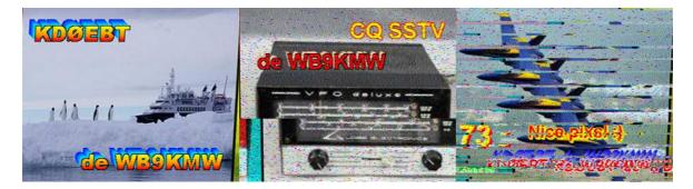
A ham will sometimes find their SSTV software hiccups during transmission. That may create a break in the image as viewed on the left. Or it may be caused by outside interference. Look closely at the picture on the right. Just past the half-way point you see noise lines. In this instance it was caused by QRM interference from the 2 meter repeater IDing!!
