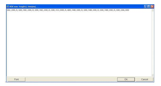
But what do they mean? Each pair to two numbers represents the frequency to be transmitted in Hertz and the duration of the transmission in milliseconds. So the pair of 392, 200 means a tone of 392 Hz, which represents the note G on the treble clef staff is transmitted for 200 ms.
